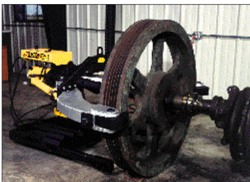
◀ The EPH-1002 quickly and easily removes this drive sheave from its shaft.
