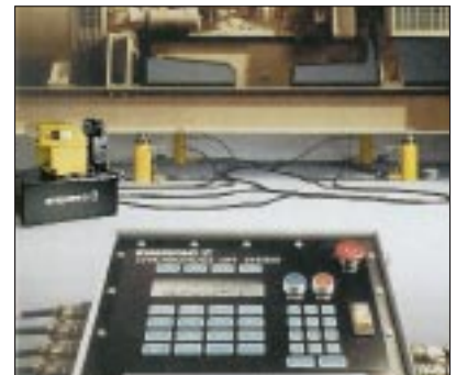
▼ Even positioning and leveling large machining centers benefits from synchronized techniques.
